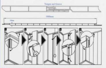
WetArea Panels feature a tongue and groove joint which provides a tight waterproof fit and an almost seamless joint between panels.
